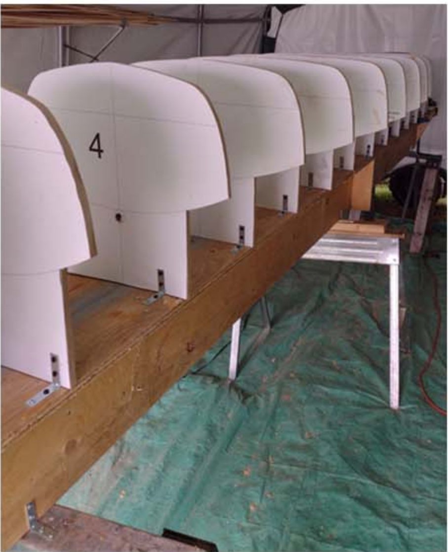
Molds set up for the construction of the first Pukaskwa 20. Photo: RHW
